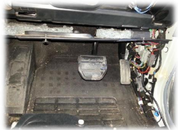
Vehicle Footwell, Right-hand Side, Panelling Removed
