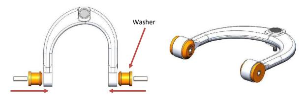
Note: Polybushes should be fitted to both upper suspension arms on both sides of the vehicle.
